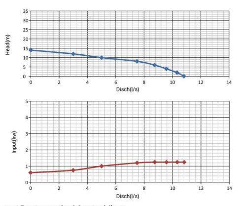
These curves are at 7 meters suction & 3 meter delivery
